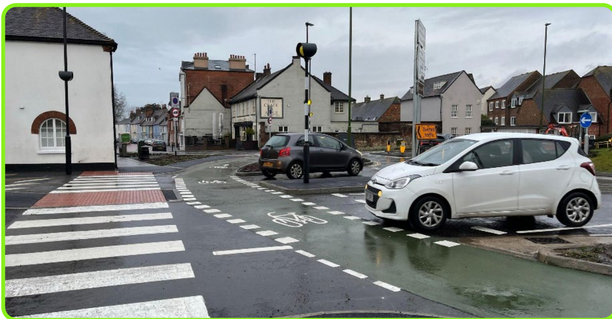
Figure 10-25: Roundabout with parallel crossings, Chichester.
