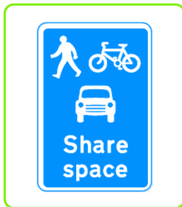
Figure 12-4: Sign to diagram 886 – road ahead where motorists, cyclists and pedestrians should expect to share the same space.
