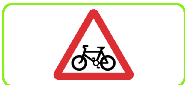
Figure 12-11: Diagram 950 – Cycle route ahead.
