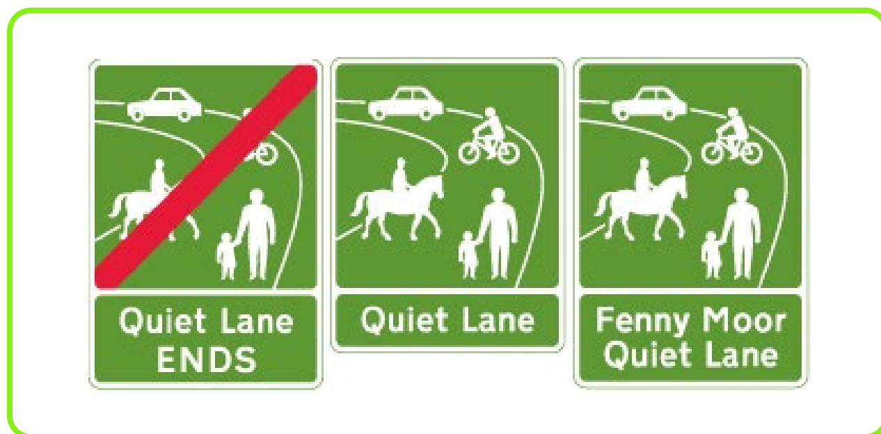
Figure 12-5: Two variations of diagrams 884 showing the start of a Quiet Lane and diagram 885 showing the end of a Quiet Lane.
